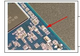
When R28 is removed, please reinsert CPU module onto DL2 PCB and reinsert DL2 PCB into JB70 Electronic unit. Reconnect all cables.
