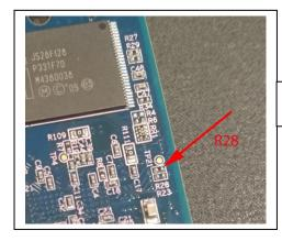
On backside of CPU unit locate R28, a surface mounted resistor.
