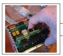
Locate and remove DL2 PCB
